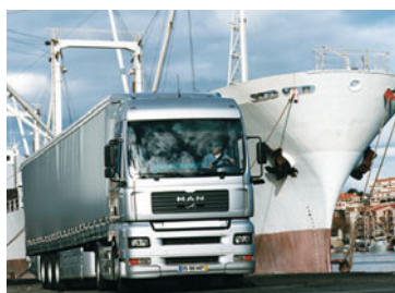
The radiator guard and the bumper corners of this massive truck are made of ABS copolymer.
